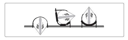
Correct way of transporting Epic **V5 or V7** on a padded roof rack with or without supporting cradles.
