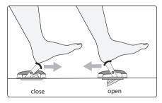
Open the bailer to drain any water out of the cockpit. Use your hand or one of your heels to push the lever back toward your body to "open" position.
